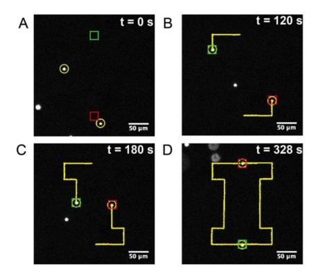
Using the Stokes Trap, the researchers can manipulate particles to follow any predetermined path. Credit: Anish Shenoy
