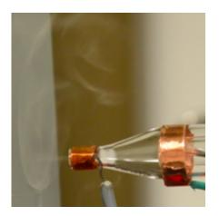
The nozzle firing a jet of carbon nanotubes with helium plasma off and on. When the plasma is off, the density of carbon nanotubes is small. The plasma focuses the nanotubes onto the substrate with high density and good adhesion. Credit: The nozzle firing a jet of carbon nanotubes with helium plasma off and on. When the plasma is off, the density of carbon nanotubes is small. The plasma focuses the nanotubes onto the substrate with high density and good adhesion.CREDIT: NASA Ames Research Center
