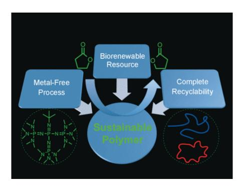
Most plastic and polymer materials around are poorly sustainable, as they are petroleum-based, their preparation needs metal catalysis, and they persist in the environment and cannot be effectively recycled. Seeking for true sustainability, American scientists have now prepared a fully recyclable biopolyester from a biofeedstock-based chemical without any metal catalyst involved. As they report in the journal *Angewandte Chemie*, the polymer is best suited for regular polyester
