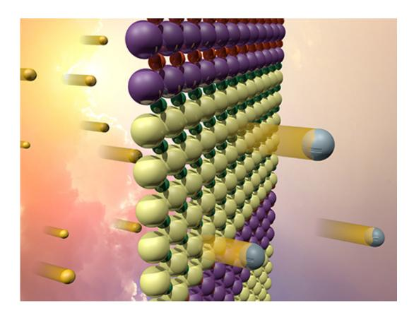
The interfaces between the two oxides (represented in this idealized, atomically abrupt model by the yellow and purple bands) create an electric field. The field separates electrons (silver) excited by sunlight (gold), which could be used to catalyze hydrogen fuel production.
