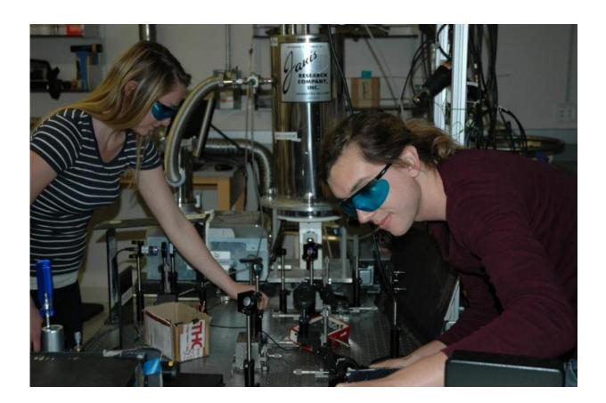
Erica Calman and Chelsey Dorow align optics required to collect measurements from a molybdenum disulfide sample. Credit: Calman
