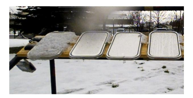
SLUGs coatings on the right three panels at a test station repel snow and ice, but snow builds up on an untreated panel (far left). Credit: Chihiro Urata
