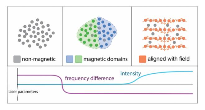
To explore magnetism in a cloud of rubidium, the JQI researchers first cooled their atoms down. Because the atoms were so cold, they inhabited only three low-lying quantum energy levels, or states. These states, labeled by a quantum property called spin, interacted differently with magnetic fields. Two of the three states tried to align with or against an applied field, while the third completely ignored it.
