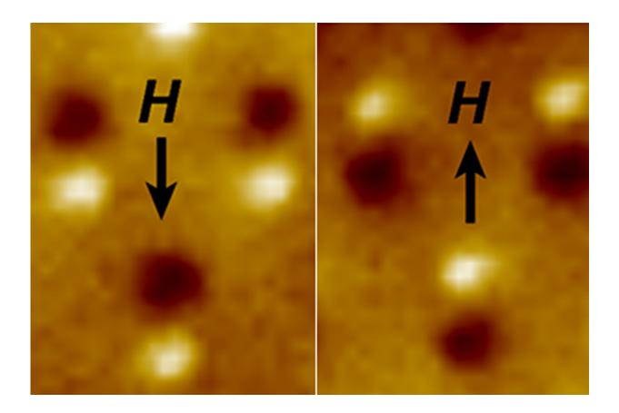
Magnetic microscope image of three nanomagnetic computer bits. Each bit is a tiny bar magnet only 90 nanometers long. The microscope shows a bright spot at the "North" end and a dark spot at the "South" end of the magnet. The "H" arrow shows the direction of magnetic field applied to switch the direction of the magnets. Credit: Jeongmin Hong and Jeffrey Bokor
