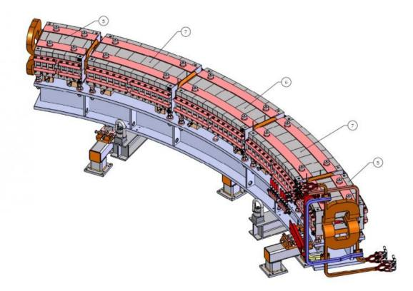
An engineering schematic of the curved magnet girder holding three full-length and two half-length magnets. After successful testing, five more will be built to the same specifications and assembled to form the ends of the prototype accelerator.
