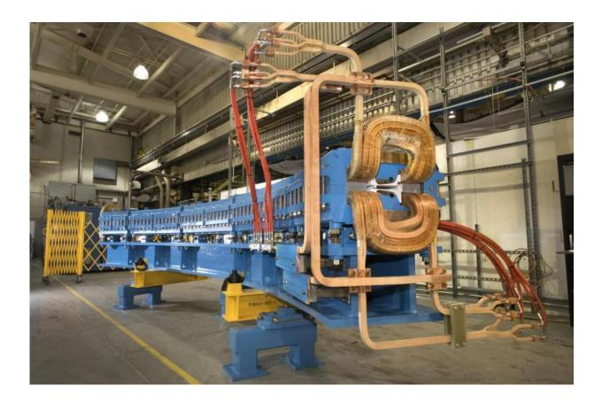
This end view of the girder shows the magnet iron in blue, and the multiple copper conductors that carry the electrical current to make the magnetic field. The conductors are contained in a block of epoxy to insulate them from each other. Cooling water flows through the center of the conductors, entering and leaving by the orange feed pipes in the background.
