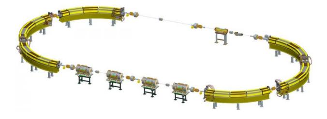
Six curved magnet girders will be incorporated into a "racetrack" shaped accelerator—three on each end for turning the beam. The straight sections will incorporate additional equipment for injecting, accelerating, and extracting the ion beams.
