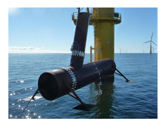
Researchers fitted a test pipe knot with two sensor ring demonstrators for practical trials in the Baltic Sea. Credit: Fraunhofer IKTS
