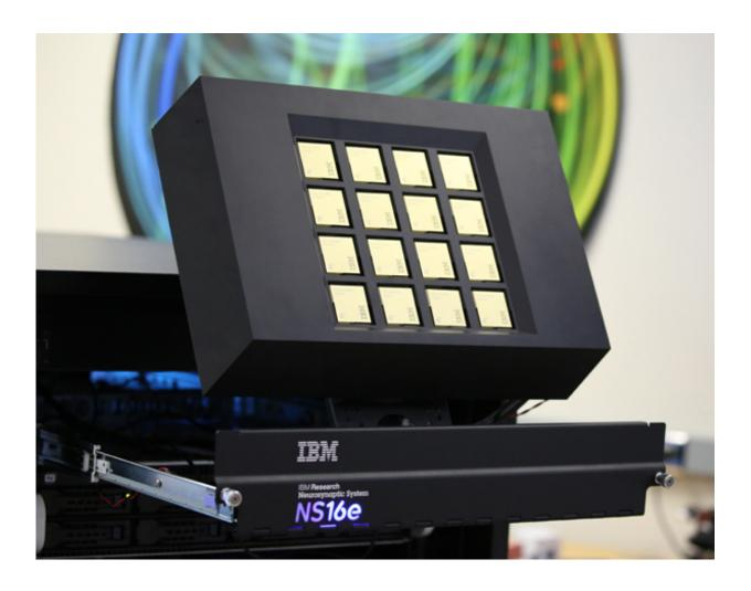
The 16-chip IBM TrueNorth platform Lawrence Livermore will receive later this week. The scalable platform will process the equivalent of 16 million neurons and 4 billion synapses and consume the energy equivalent of a hearing-aid battery – a mere 2.5 watts of power. Photo courtesy of IBM.
