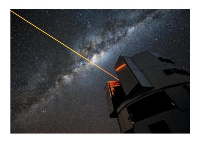
A 22W laser used for adaptive optics on the Very Large Telescope in Chile. A suite of similar lasers could be used to alter the shape of a planet's transit for the purpose of broadcasting or cloaking the planet. Credit: ESO / G. Hüdepohl
