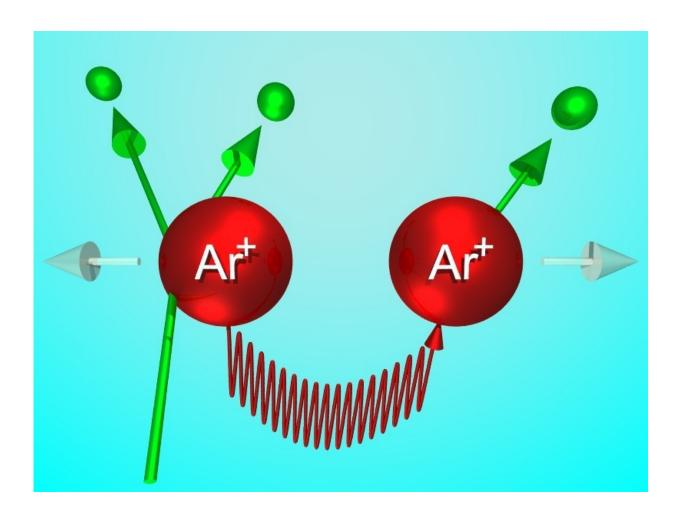
Protocol of a decay process: When an electron collides with an argon atom in a two-atom molecule (left), it knocks out a secondary electron and is deflected from its orbit as a result. The argon atom absorbs energy and transmits it to the other atom (red zigzag line). This atom is also ionized and the two argon ions repel each other. Two additional slow electrons arise in the process. The harmful impact of electron radiation, as arises in the case of radioactive beta decay, is
