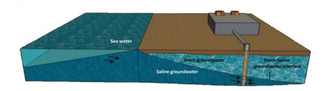
A diagram showing where saline groundwater is extracted for desalination
