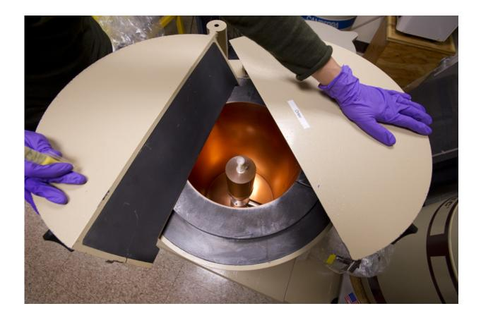
Prepared sample from Fukushima being inserted into lead-lined gamma well detector. Credit: Tom Kleindinst, Woods Hole Oceanographic Institution
