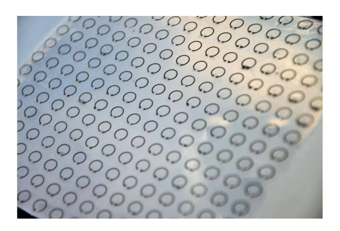
This flexible, stretchable and tunable "meta-skin" can trap radar waves and cloak objects from detection. Credit: Liang Dong/Iowa State University
