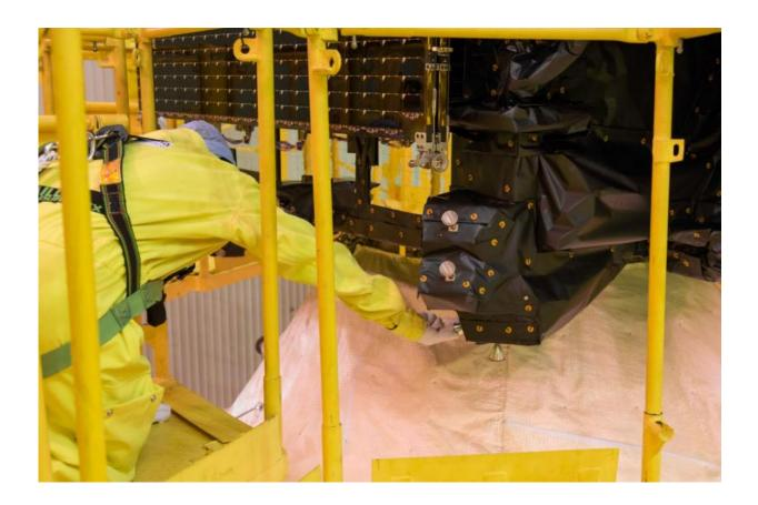
Protective covers are being removed from the thrusters on the Trace Gas Orbiter, before the spacecraft is encapsulated within the launcher fairing. Credit: ESA - B. Bethge
