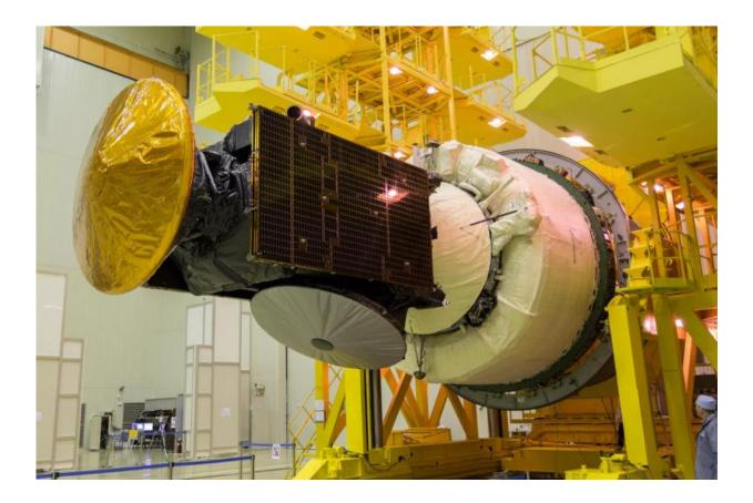
The ExoMars 2016 spacecraft composite, comprised of the Trace Gas Orbiter and Schiaparelli, mated with the Breeze upper stage on the launch vehicle adapter, ready for encapsulation within the launcher fairing. Credit: ESA - B. Bethge
