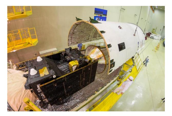
The ExoMars 2016 spacecraft composite, comprised of the Trace Gas Orbiter and Schiaparelli, seen during the encapsulation within the launcher fairing. The conical shape to the left is the launch vehicle adapter, through which the spacecraft is attached to the Breeze upper stage. The first half of the fairing has already been rolled into place underneath the spacecraft assembly, and the second fairing half is being manoeuvred into place by means of an overhead crane. Credit: ESA - B. Bethge
