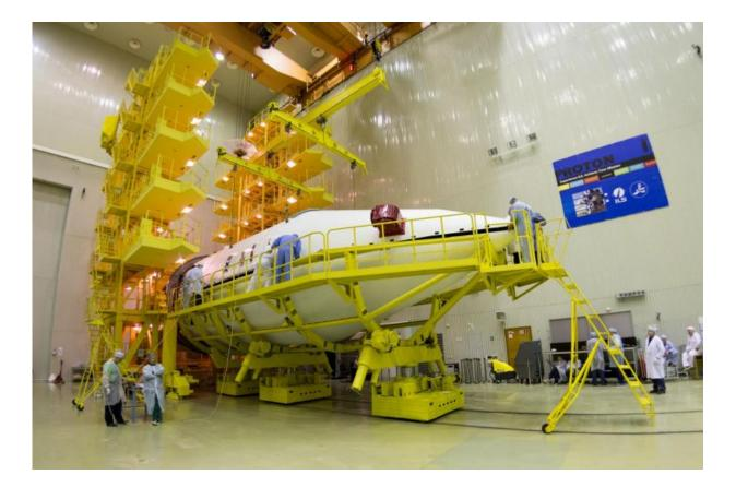
The ExoMars 2016 spacecraft composite, comprised of the Trace Gas Orbiter and Schiaparelli, seen during the final stages of encapsulation within the launcher fairing. The first half of the fairing had already been rolled into place underneath the spacecraft, and the second fairing half is being lowered into place by means of an overhead crane. Credit: ESA - B. Bethge
