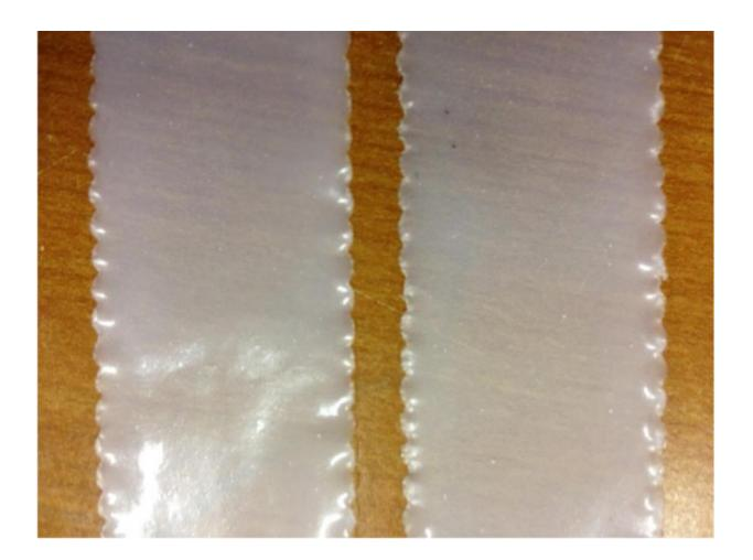
Adding eggshell nanoparticles to a bioplastic (shown above) increases the strength and flexibility of the material, potentially making it more attractive for use in the packaging industry. Credit: Vijaya Rangari/Tuskegee University
