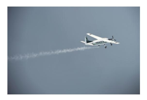
An aircraft from the Thai Department of Royal Rainmaking deposit a sodium chloride-based material above clouds in Nakhon Sawan in an effort to produce rain
