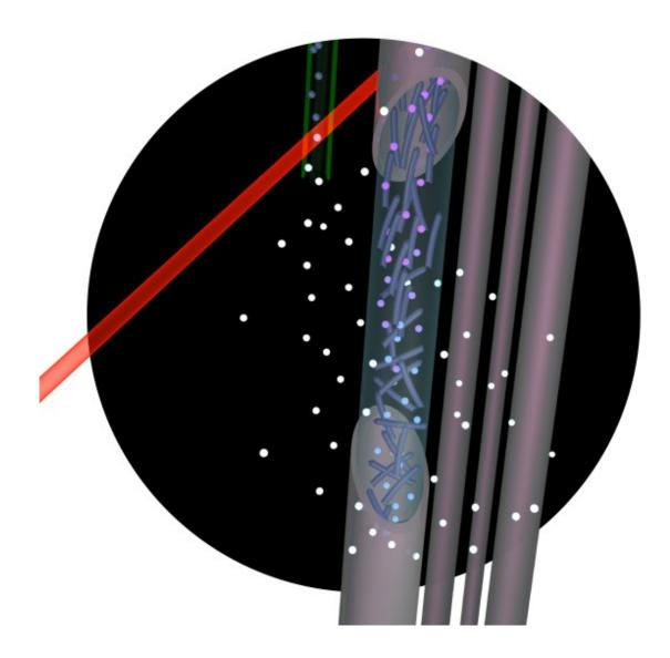
This illustration shows how the new method works. Hyperpolarized xenon-129, which can sense molecular ordering within samples, diffuses through hollow membrane fibers containing viscous liquids. Different chemical environments,
