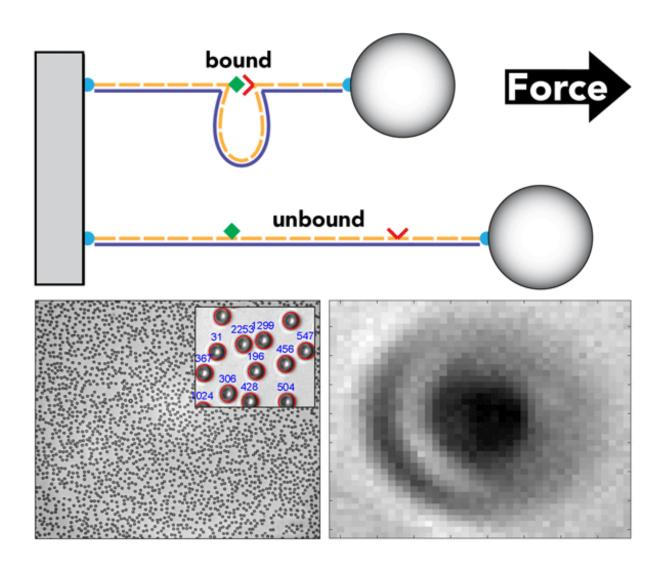
The picture on the top shows a DNA nanoswitch that forms a looped structure
