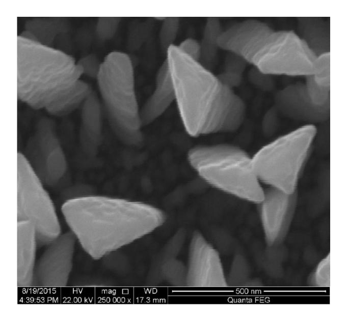
Nanostructures fabricated with iron oxide and titanium dioxide are seen magnified to 250,000 times their actual size. Research led by Kun Yao, a faculty
