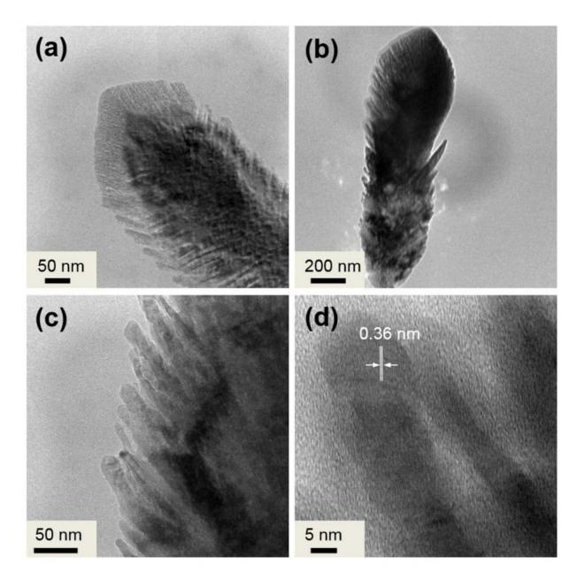
This cross-section view of the nanostructures shows a darker inner core of iron oxide coated with a layer of titanium dioxide.
