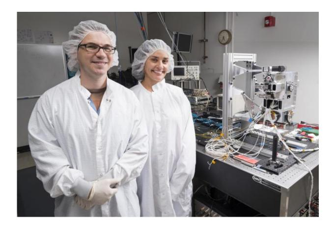
JPL's David Aveline and Anita Sengupta are seen with the physics package for the Cold Atom Laboratory, which includes a vacuum chamber where ultra-cold quantum gases are made. Credit: NASA/JPL-Caltech
