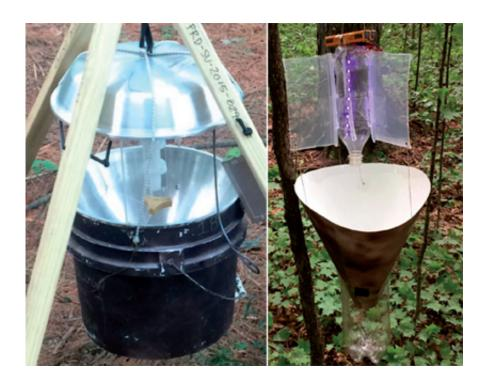
Twelve-volt mercury vapor black light traps like the one on the left are heavy and cost between 200-500 dollars apiece. The new LED funnel trap (right) is lightweight and costs about \$28.50. Credit: Entomological Society of America
