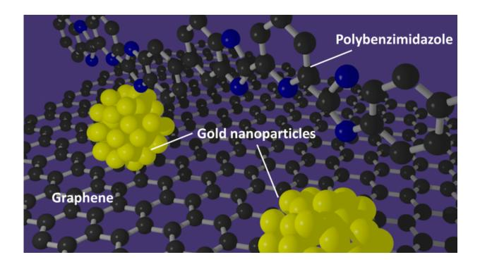
A polybenzimidazole polymer supports the formation of gold nanoparticles with well-defined sizes on graphene. Credit: International Institute for Carbon-Neutral Energy Research (I<sup>2</sup>CNER), Kyushu University
