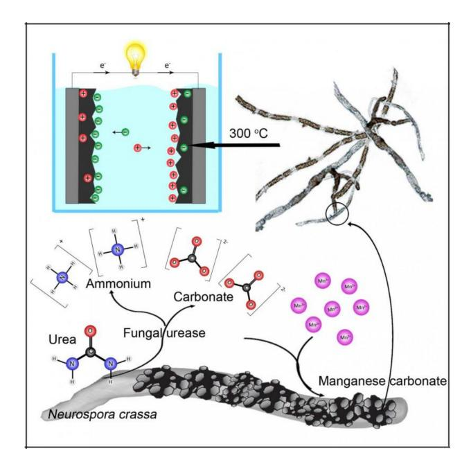
This graphical abstract depicts how Li and Gadd *et al.* synthesized novel electrochemical materials using a fungal Mn biomineralization process. They studied the electrochemical properties of the carbonized fungal biomass-mineral composite in a supercapacitor and a lithium-ion battery, thus providing a novel biotechnological method for preparation of sustainable electrochemical materials. Credit: Li and Gadd *et al.*/*Current Biology* 2016
