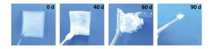
Photographs from BD-TENG at various stages of the degradation time line suggest that devices encapsulated in PLGA were initially resistant to mass degradation. However, after 40 days, significant mass loss and structure disintegration was initiated. Near-total mass loss was observed at 90 days. Credit: *Science Advances* (2016). DOI: 10.1126/sciadv.1501478
