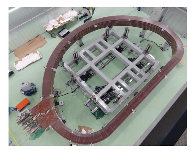
iew of Europe's first winding pack, the inner-core of a Toroidal Field coil, which will magnetically confine ITER's plasma. ASG Facilities, February 2016. Credit: F4E
