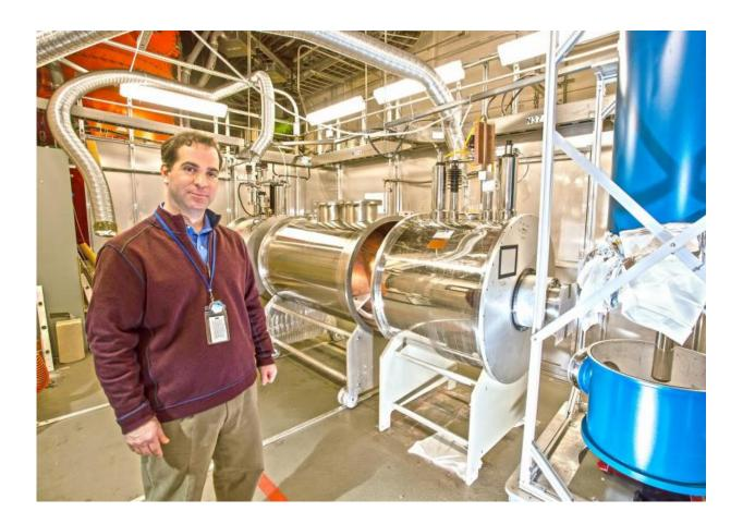
Princeton physicist Chris Tully in the PTOLEMY laboratory at PPPL. Behind him are powerful superconducting magnets on either side of the vacuum chamber. Credit: Elle Starkman/PPPL Office of Communication
