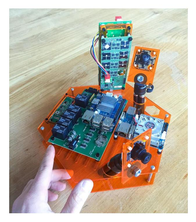
Inside each node is a set of computing hardware and environmental sensors comprising the Waggle smart sensor platform, developed by scientists at Argonne National Laboratory. The sensors use lasers to "count" airborne particulates and determine their size as they cross the laser light's path.
