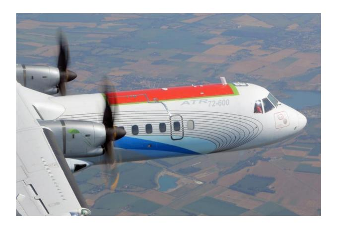
The test aircraft was a medium-range model for about 70 passengers. For flights, a CFRP component which was about five-by-three-meters long was used. This area is one of the most heavily stressed components during flight. Credit: Alenia Aermacchi
