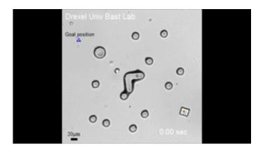
By responding to the way electric fields deform around static obstacles, bacteriapowered microrobots using Drexel's algorithm can detect the obstructions and adjust their course.
