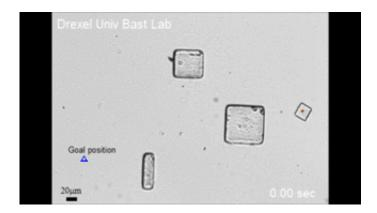
Drexel researchers have developed a method for using electric fields to help microscopic bacteria-powered robots detect obstacles in their environment and navigate around them to get to their destination.
