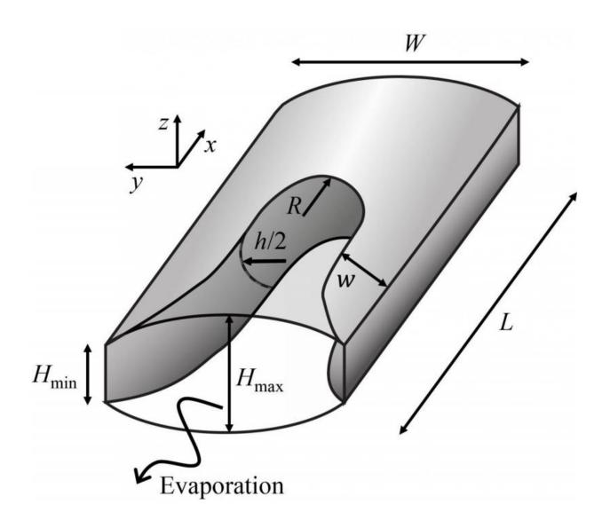
A glass channel with a rectangular-like cross section closed at one end and open
