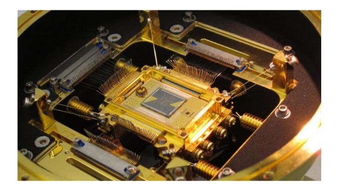
The heart of the ASTRO-H Soft X-ray Spectrometer is the microcalorimeter
