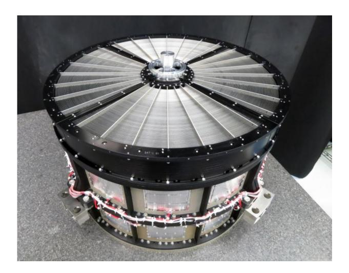
The Goddard team provided identical mirror assemblies for both of the Soft Xray Telescopes aboard ASTRO-H. Each is 17.7 inches (45 centimeters) across and contains 1,624 precisely aligned aluminum mirror segments arranged in 203 concentric shells. Credit: NASA's Goddard Space Flight Center
