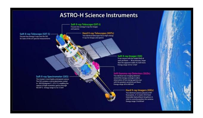
This illustration shows the locations and energy ranges of ASTRO-H science instruments and their associated telescopes. One keV equals 1,000 electron volts, which is hundreds of times the energy of visible light. Credit: JAXA/NASA's Goddard Space Flight Center
