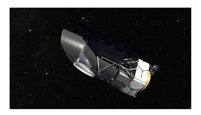
NASA's Wide Field Infrared Survey Telescope (WFIRST), illustrated here, will carry a Wide Field Instrument to capture Hubble-quality images covering large swaths of sky, enabling cosmic evolution studies. Its Coronagraph Instrument will directly image exoplanets and study their atmospheres. Credit: NASA/GSFC/Conceptual Image Lab
