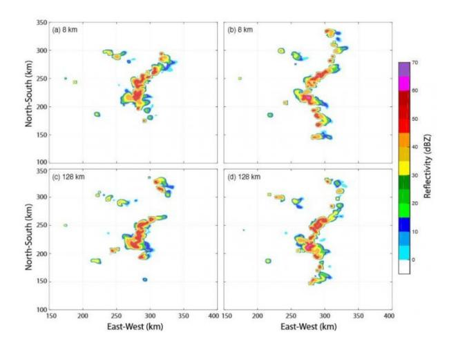
Simulated radar images from two thunderstorms. The top panels included initial errors at the 8-km horizontal scale, but give similar results to the bottom panels, which had more minor errors, only a quarter the size, at the larger 128-km scale. Credit: Dale Durran/University of Washington
