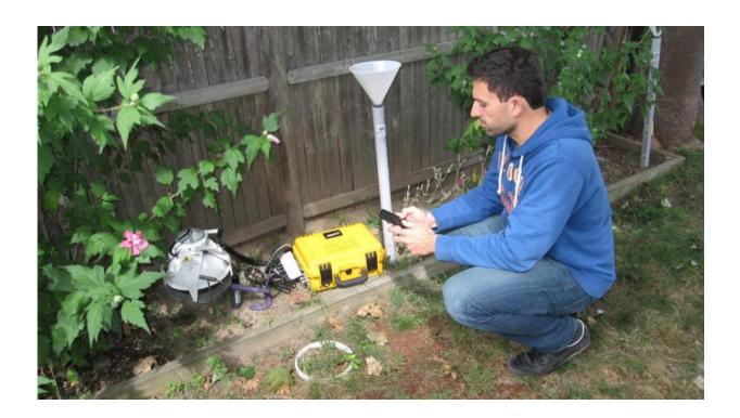
Stephen Decina, Boston University PhD student, measures carbon dioxide being released from the soil using an automated soil carbon dioxide efflux system. The equipment, which is controlled with a smartphone, passes air through an infrared gas analyzer and measures the concentration of carbon dioxide accumulation over time. Credit: Stephen Decina
