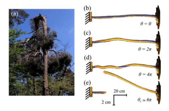
Breakage induced by torsion. (a) A tree broken after a trunk torsion. (Photograph: Keraunos, Fontainebleau forest, France, June 2010). (b)–(e) Snapshots from experiments. Wood rod of length L=900 mm and diameter D=4 mm. Snapshots are stretched vertically to emphasize the deformation out of its axis (note the two scale bars). Credit: (c) *Physical Review E* (2016). DOI: 10.1103/PhysRevE.93.023001
