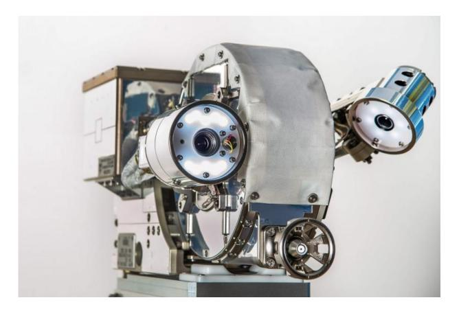
On Oct. 9., 2015, NASA used the zoom lens (left) on VIPIR, a new inspection space tool, to examine an unexplained discoloration on the SSRMS, the Space Station Remote Manipulator System. Credit: NASA/Chris Gunn
