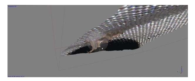
The Image Science and Analysis Group at Johnson is continuing to analyze the results from VIPIR's inspection. 3D models (as shown in this GIF), built from VIPIR imagery and supplemental data, are helping the team better understand the raised mass on the space station's arm. Credit: NASA/JSC – Image Science and Analysis Group
