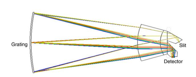
JPL researchers report in Optical Engineering on a new imaging spectrometer design to improve Landsat images. Above, Fig. 3: Spectrometer ray-trace in the spectral direction. The two reflecting prisms and planoconvex element are made of CaF2. The grating aperture as shown is 14 cm in diameter. Credit: Pantazis Mouroulis, JPL, et al.
