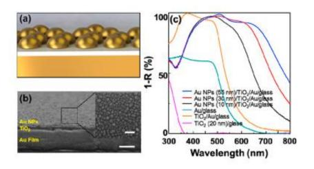
Two-dimensional metastructured film with Titanium Oxide is fabricated as a photo-catalytic photoanode with exceptional visible light absorption. Credit: UNIST
