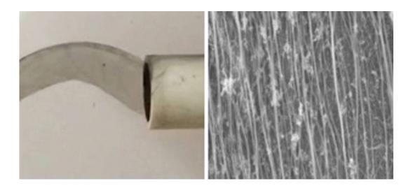
(Phys.org)—A new technique developed by researchers at East China University of Science and Technology and Shanghai Jiao Tong University has led to the development of a high-strength carbon nanotube film that retains much of the elasticity of native carbon nanotubes. In their paper published in the journal *Nano Letters*, the team describes their technique and the characteristics of the materials they made.
