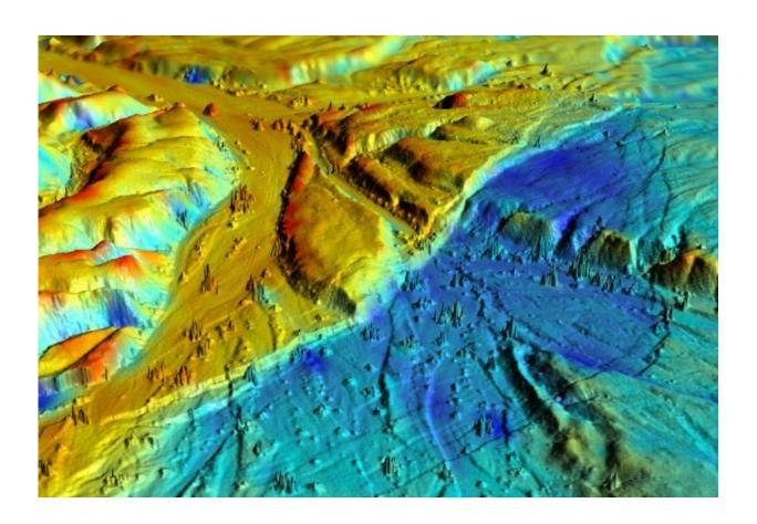
This 3-D LiDAR imaging of the Borrego Fault, ruptured during the 2010 El Mayor-Cucapah earthquake in Baja California, Mexico shows numerous small faults. The various colors represent elevation changes during the earthquake. Credit: UC Davis
