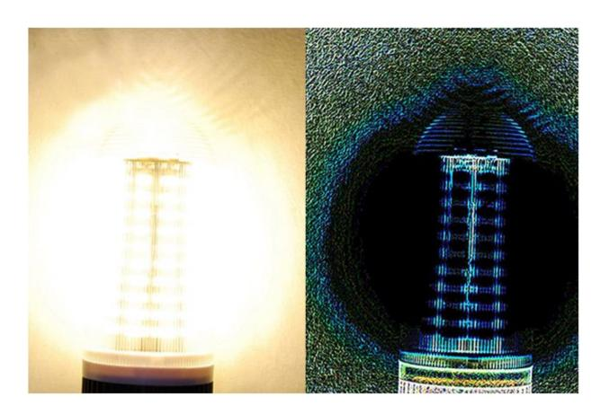
An LED light (left) and an image of the same light produced using the Phase Stretch Transform-based algorithm. Credit: Bahram Jalal
