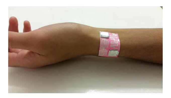
The Paper Skin sensor performs as well as other artificial skin applications currently being developed, while integrating multiple functions using cost-effective materials. Credit: KAUST
