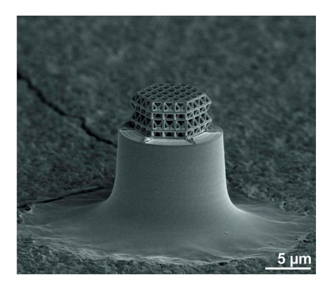
The smallest lattice in the world is visible under the microscope only. Struts and braces are 0.2  $\mu$ m in diameter. Total size of the lattice is about 10  $\mu$ m. Credit: J. Bauer / KIT
