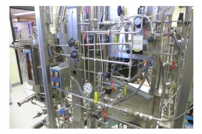
Feed ports, valves, gauges and apparatus needed to control the fermenter at left. Credit: David Tenenbaum
