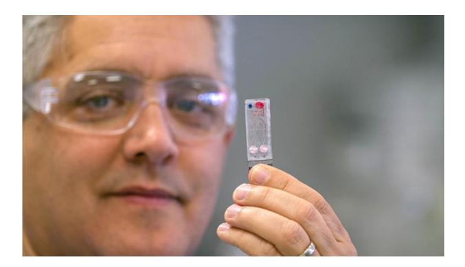
Radiobiologist Matt Coleman displays a passive flow lateral device for biodosimetry developed at Lawrence Livermore National Laboratory. It's a single use protein detection assay similar to the medical diagnosis instrument Coleman helped develop for NASA for use in deep space. Credit: Julie Russell
