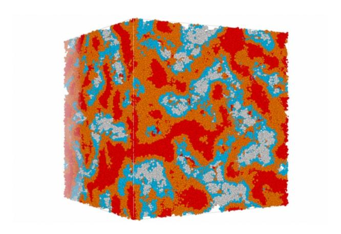
This image of a simulated concrete sample shows the "packing fraction" which describes the fraction of the volume that is filled with solid material. In this case, the average packing fraction is 0.52. Colors indicate the variations within the sample, ranging from less than 0.4 to more than 0.64. The size of the cube is 0.6 microns (millionths of a meter).
