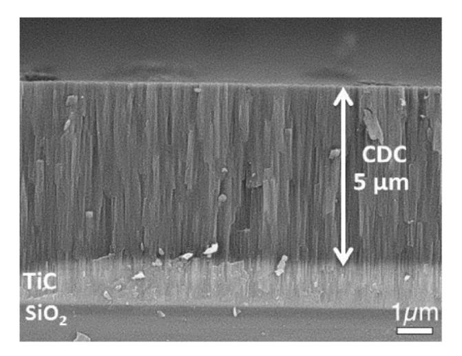
Layered structure of the carbon films on silicon chips. Credit: A. Demortiere/LRCS
