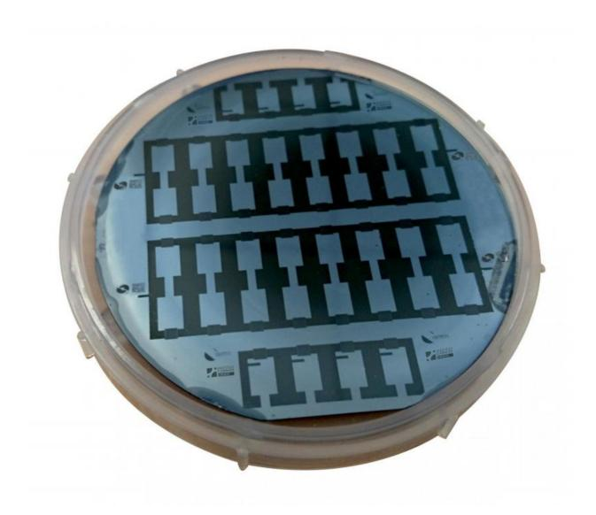
A silicon wafer containing 40 micro-supercapacitors. Credit: Lethien/IEMN
